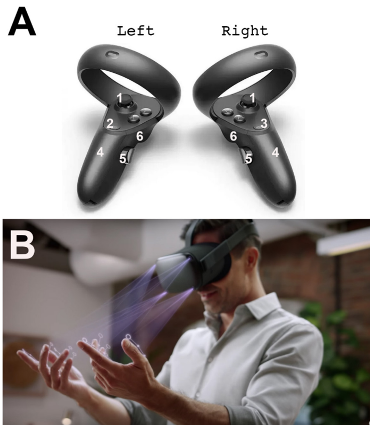
Figure 2. (A) Oculus Quest controller (1: Thumbsticks, 2: Menu Button, 3: Oculus Button, 4: Battery Covers, 5: Grip Buttons, 6: Triggers), (B). Front Facing Cameras
